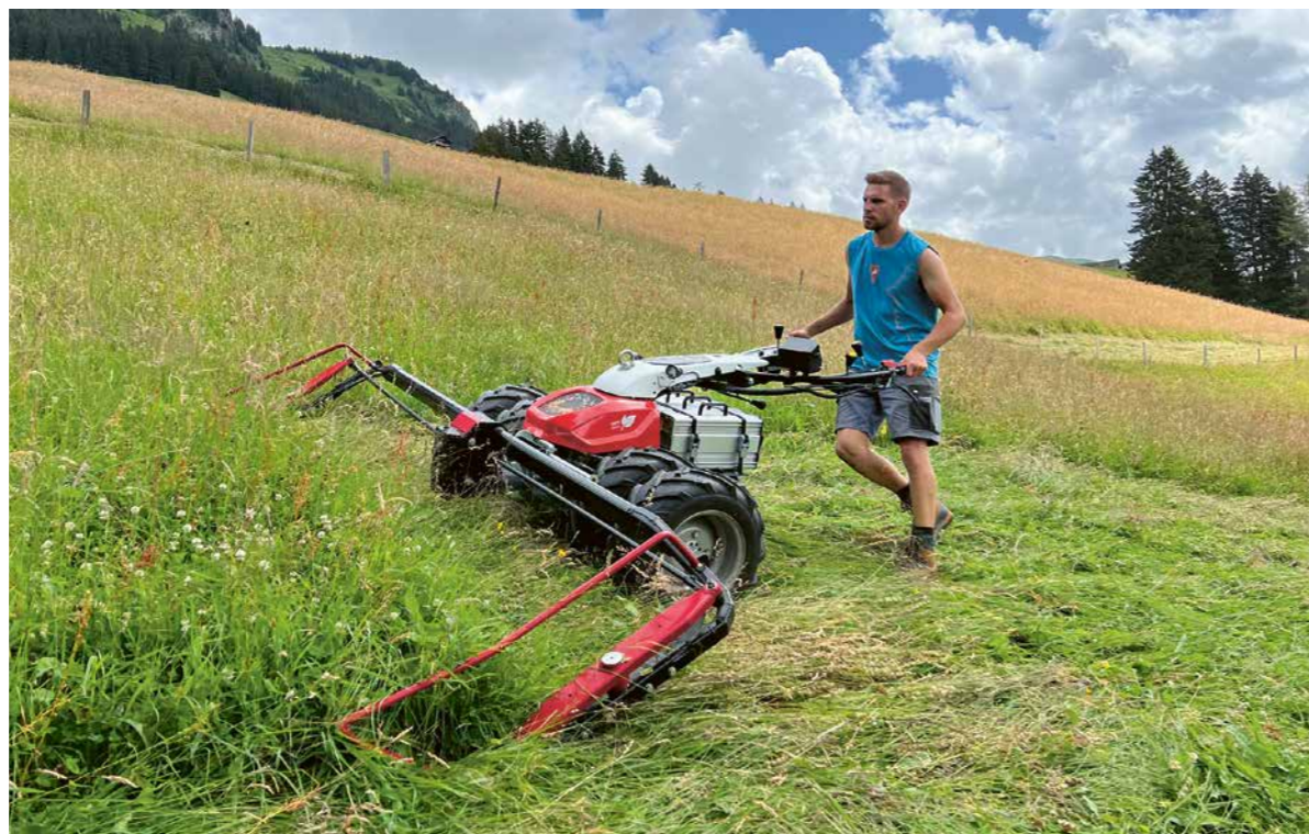
Aebi CC 140e: The popular, versatile single-axle implement carrier from Aebi is now also available with electric drive.
