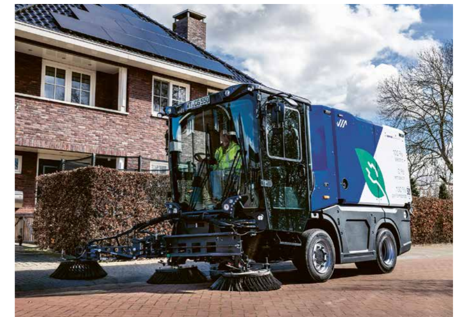
Electrically driven machines on the rise: an electric-hydraulic Nido eSyntos (above) and the new Schmidt eCleango 550 compact sweeper (right).
